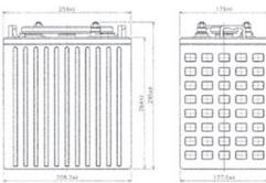
6V 260 Ah at 20 houres discharge З ca. 33.0 kg +/- 3% 6.50 - 6.70V Discharge: Charge: Storage:  $0^{\circ}C - 50^{\circ}C$ - 20°C – 60°C - 20°C – 60°C 20°C ± 5°C Valve Regulated Lead Acid (VRLA) batteries can be stored for more than 3 months at 20°C. Please charge batteries before using. Dual Fit
