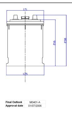
**PERFORMANCES** Voltage (V): 6 V C20 (Ah): 140.0 20 h 900 ΕN Cranking (A): WET Charge: Vented/Flooded Technology: Grid: Hybrid Vibration: V3 (30Hz+/-2Hz/6g/20h)
